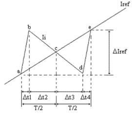
Fig. 1. Input current profile within a switching period.
