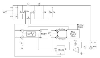
Fig. 4. Proposed controller associated with a boost converter.
