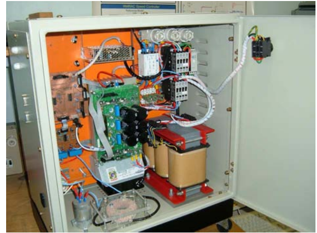
Fig. 2. The designed AC power source
