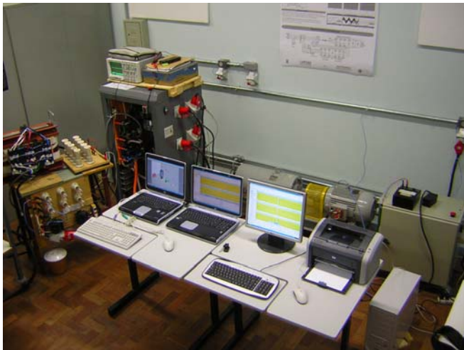
Fig. 12. The reduce scale laboratory prototype - 5kVA DFIG
