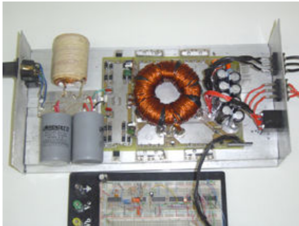
Fig. 20. Prototype developed of the inverter
