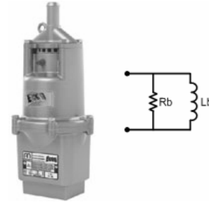
Fig. 1. Pump equivalent electrical model.
