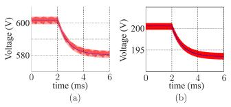
Fig. 15. Simulation results for the switching model (in red) and deduced transfer function (in blue) for a negative step of 3% in duty cycle from nominal condition a) in an IPOS association (10 V/div and 2 ms/div); b) in an IPOP association (5 V/div and 2 ms/div).
