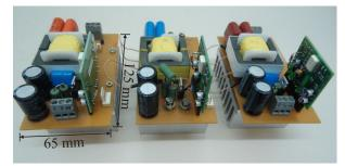
Fig. 9. Prototype composed of 3 Flyback modules.
