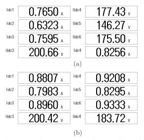
Fig. 13. Test 1 - Wattimeter measurements for an a) IPOS association (Full load); b) IPOP association (Full load). Idc1, Idc2, Idc3 - Average input current values on modules 1, 2 and 3, respectively. Udc4/Idc4, Udc5/Idc5, Udc6/Idc6 - Average output voltage/current values on modules 1, 2 and 3, respectively. Udc3 - Average input voltage.
