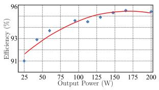
Fig. 12. Efficiency of one module for an IPOP association. The pointed blue line represents the experimental results and the continuous red line the trend curve.
