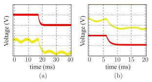
Fig. 16. Experimental (yellow) and simulated (red) a) IPOS converter output voltage dynamics for a negative step of 0.02 in duty cycle (30 V/div); b) IPOP converter output voltage dynamics for a negative step of 0.02 in duty cycle. (10 V/div).
