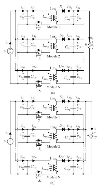
Fig. 1. IPOS (a) and IPOP (b) modular Flyback connections.
