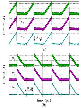
Fig. 11. Experimental a) primary side current in an IPOP (2 A/div); b) secundary side current in an IPOP (2 A/div).
