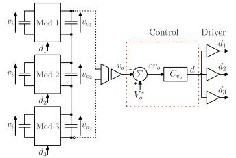
Fig. 8. Simplified control diagram for three modules in an IPOS connection.
