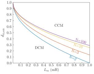
Fig. 3. Critical duty cycle value of one module to guarantee its operation in DCM based on the number of modules N and the magnetizing inductances  $L_m$ .
