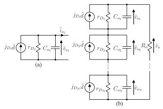
Fig. 6. Equivalent secondary-side small signal model a) for a single module; b) for an IPOS association.
