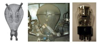
Fig. 1. Mercury Arc Valve (Rectifier): The original prototype by P. C. Hewitt in 1902 (left) and an old industry product (center) and a more recent RC85 thyratron [7, 8].
